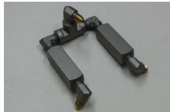
11. High Pressure Check Valve Assembly
