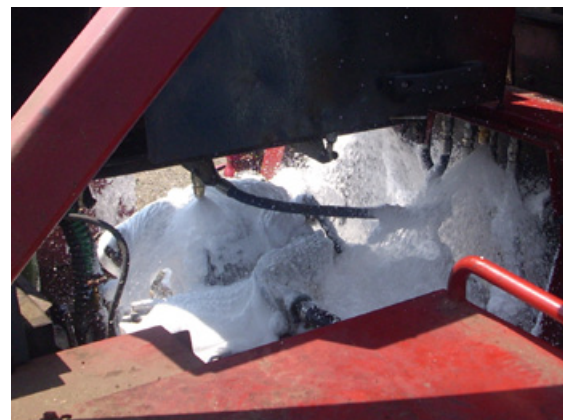
Engine and hydraulic compartment protection. Tyler Big Red 48K Fork Lift
